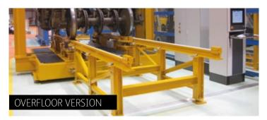
Bogies must be placed onto the test stand by crane for loading and the later unloading. The integration into a client's assembly line is possible.
