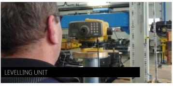
For height measuring and calibration of the system.
