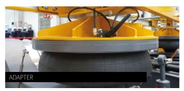
This is the mechanical interface between load application and the bogie. A very important bogie-specific component for an accurate load application.
