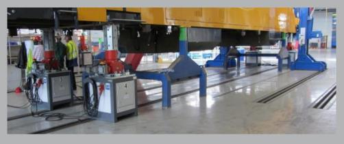
Determination of the load which the vehicle body applies onto the bogie
