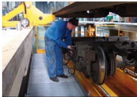
LOWERING SYSTEM WITH CHAIN PLATFORM ALLOWS EASY ACCESS DURING ASSEMBLY OF THE BOGIES.
