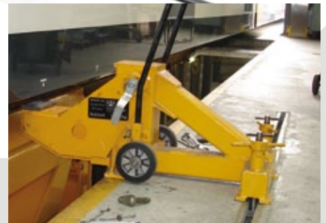
CART SUPPORT MOBILE: WELL-TRIED AND SIMPLE PRINCIPLE FOR CAR SUPPORT
