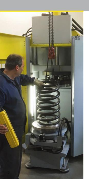
More than 90 % of tested, used springs still fulfil the test values specified by the manufacturer, even after a long period. They can be reused after a test took place.
