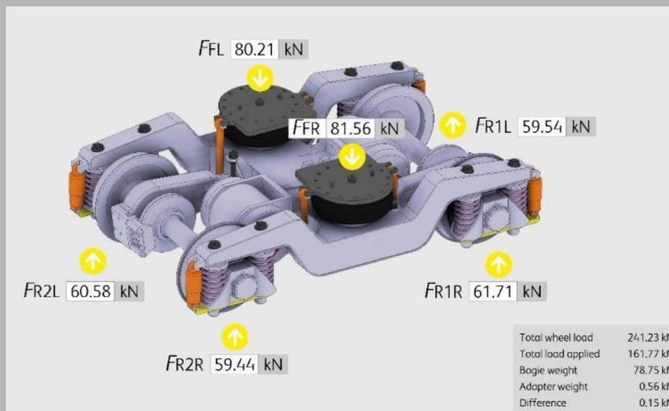
Under load simulation, it is also possible to adjust the correct heights of antenna, emergency brakes, coupling heights, etc. The DIN standard 25043-7 is a useful guideline, already considered in bogie workshops outside Europe. Regarding the wheel load the height of top of secondary suspension (bogie loading point) over T.O.R is be most important. Some rolling stock suppliers request in the their manuals < 2 mm, similar shall be between front an rear bogies.
