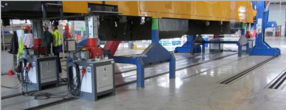
Determination of the load which the vehicle body applies onto the bogie
