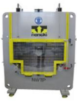
The Nencki test press is for proving that the welds are within the permitted tolerances and the rails are in accordance with the safety requirements. The test piece can easily be lifted onto the supports by crane and then shifted manually into the machine. All necessary steps are released and supervised by a PC control.
