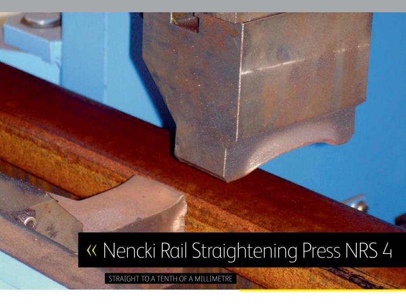
The Nencki rail straightening press is used for straightening rail profiles after the flash butt welding process. After removing the weld burr by the rail grinding machine, the rail is moved to the straightening press. The rail joint is straightened by two hydraulic cylinders in horizontal and vertical direction. The process meets the latest standards.
