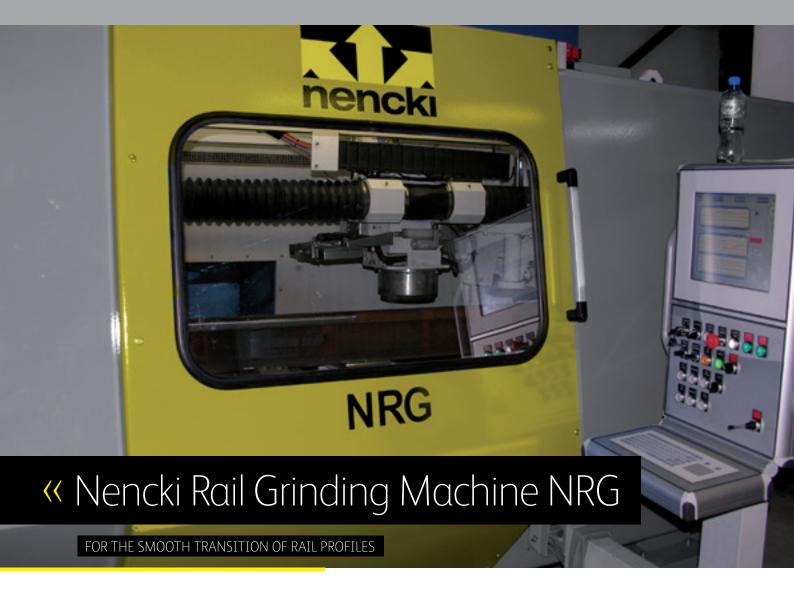
The Nencki rail grinding machine is for grinding the welded rail joint after the flash butt welding operation. The grinding is carried out on top as well as on the sides of the rail head. The process meets the latest standards. Semi- and fully automatic version featuring video camera supervision.
