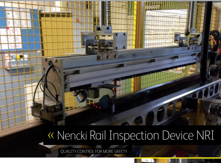
The rail inspection system of Nencki is for checking the straightness of rails at the end of a rail welding line. This control ensures that the dimensions are within the permitted tolerance and meet the required safety standards.
