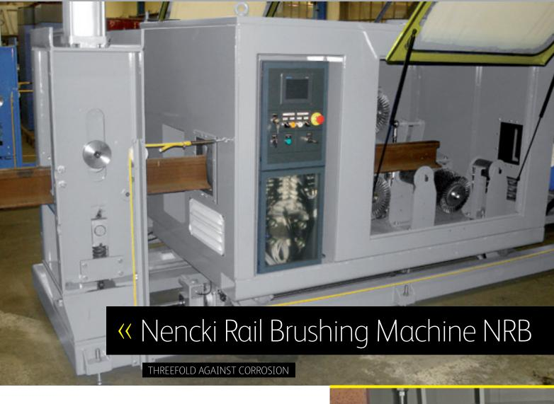
The Nencki rail brushing machine is for the preparation of rails for the flash butt welding process. Corrosion and other impurities are being removed at two rail ends in a single step. The top and bottom surfaces of the rail are cleaned in order to achieve a perfect electrical contact for the welding electrode. The front area is also cleaned by a separate brushing unit.
