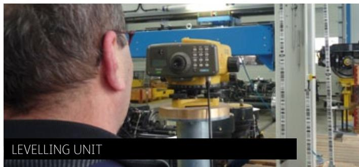
For height measuring and calibration of the system.
