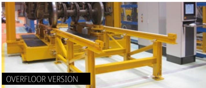
Bogies must be placed onto the test stand by crane for loading and the later unloading. The integration into a client's assembly line is possible.
